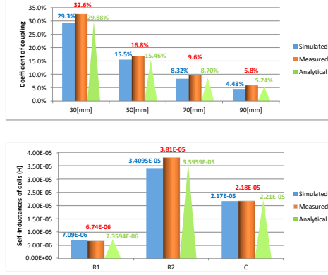
Figure 3.16: Coupling coefficient of rectangular pads at various z-gaps and self-inductances of air-cored charge pads of various shapes. The coupling is measured at various z-gaps at the best aligned point. The parameters of the coils are as presented in Table 3.2.
