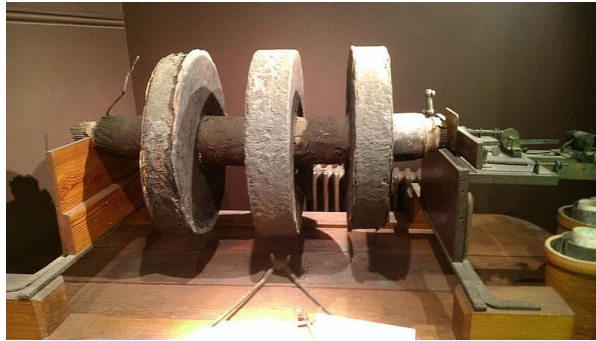
Figure 2.2: Callan's induction coils, produced sparks upto 15 inches (38.1 cm) and helped Callan recognize that induction depended on the rate of interrupting the circuit. This achievement was unchallenged till 1890 [35], [36].
