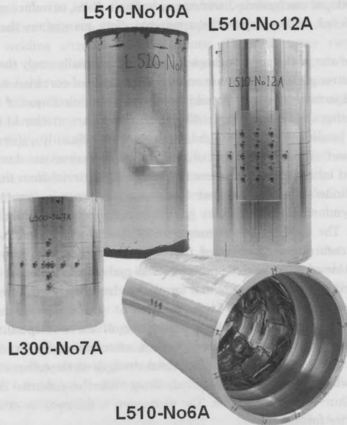
Figure 39: Photographs of typical test specimens. Clockwise from middle-left: L510-No10A, with Patch C general corrosion, after collapse testing; L510-No12A, with Patch D general corrosion, before testing; the intact specimen L510-No6A, showing the internal ring-stiffeners and strain gauge wiring, before testing; and L300-No7A, with Patch A corrosion damage, before testing.
