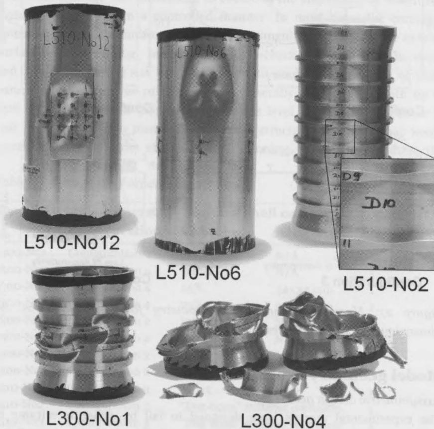
Figure 26: Typical cylinder models, before and after collapse testing. Clockwise from top-left: L510-No12, an internally-stiffened cylinder with a large patch of corrosion thinning, after volume-control testing; L510-No6, an intact internally-stiffened cylinder after volume-control testing, showing interframe dimples superimposed on an overall collapse mode; L510-No2, before testing, showing dog-bone stiffener corrosion at inset; L300-No4, a short cylinder with heavy stiffeners and a small patch of shell corrosion, showing the specimen after testing with a conventional apparatus; L300-No1, a short intact cylinder failing by interframe collapse, and showing the specimen after testing with a volume-control apparatus.
