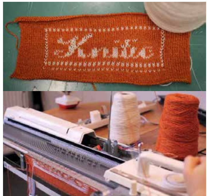
Figure 2. KNITIC digital design knitting machine & pattern example
