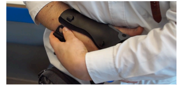
Figure 42 During the interview with Jasper a test was done with a set of different, existing, braces. It was found that Jasper used his body as an extra resting point for stability
