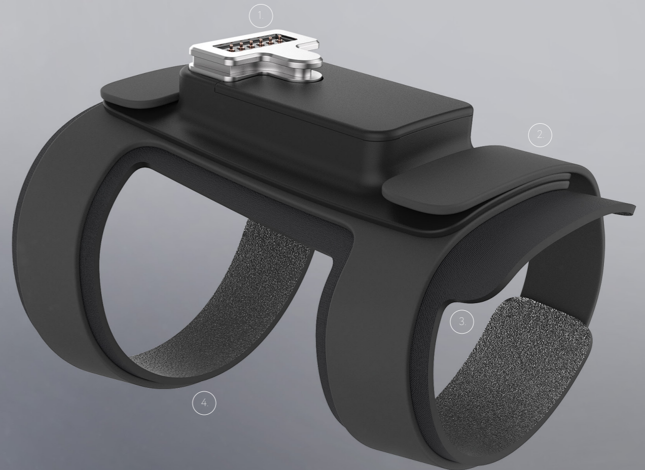
Figure 33 The final brace concept. This image is the result of the findings from the conceptual face. This 3D model has been used as the starting point of the ergonomic validation and functional tests. Added improvements have been numbered: 1. A functional force sensor design that can be easily attached to the exshell. 2. A easy to use ergonomically placed closing and opening mechanism. 3. Extra padding added on locations that need extra care 4. Laminated design to provide a balanced solution between stiff, flexible and soft materials.
