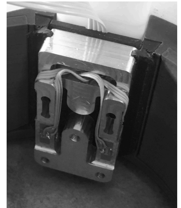
Figure 39 The cables from the force sensor have been guided from the sides of the sensor to the bottom of the pcb that contained the pogo pins.
