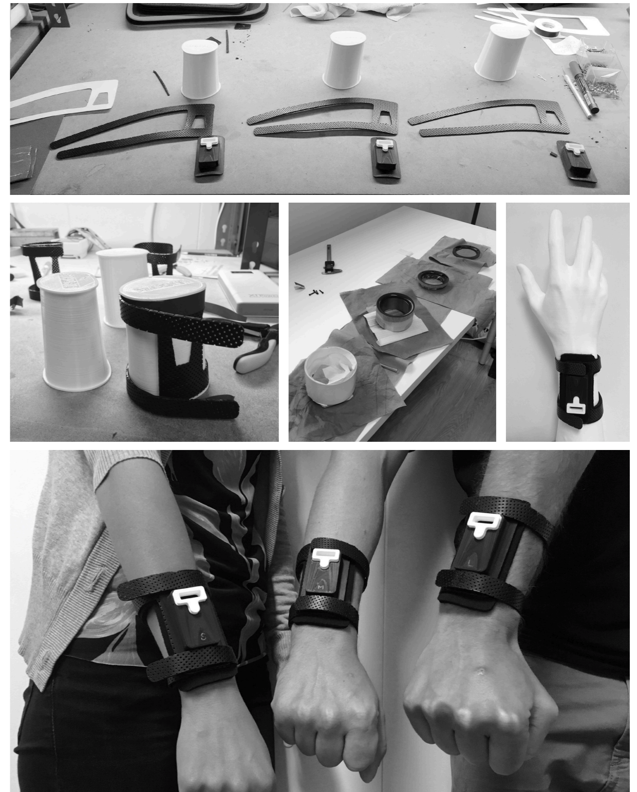
Figure 48 Some snapshots of the prototyping process. for the ergonomic prototypes used for ergonomic tests. A set of special moulds (top photo) have been made to shape the thermoplastic into the desired sizes. The results are shown on the photo on the bottom.
