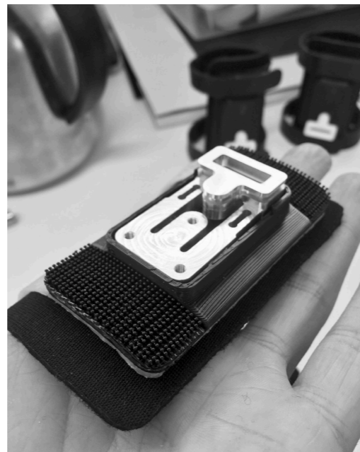
Figure 49 Making process of the functional prototype. The pcb's have been developed by de Jong (2019), other parts of the force sensor have been made in collaboration with the PMB workshop at the faculty of Industrial Design and at the workshop of STIL.
