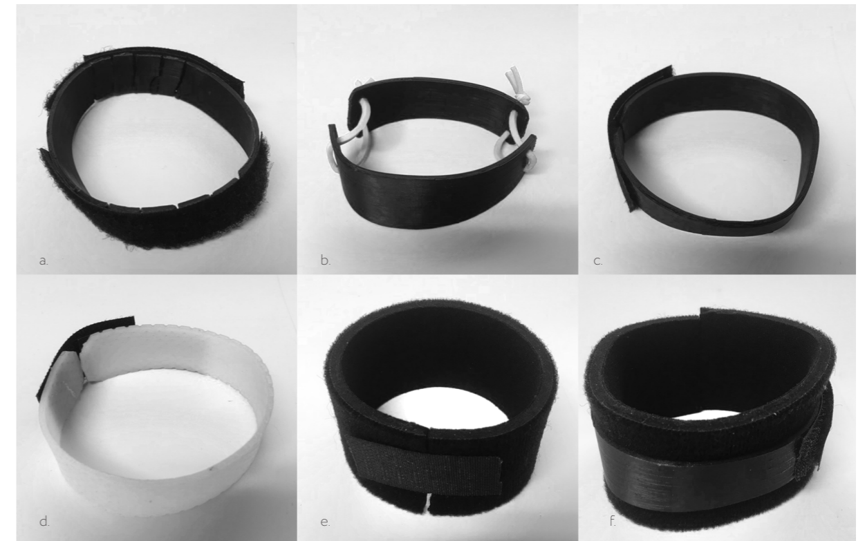
Figure 28 A set of six different types of enclosures around the wrist has been made. Each one of them was designed to test different material behavior. A. Stiff plastic combined with flexible fabric. b. Stiff plastic with flexible material on the edges of the wrist. c. fully enclosed stiff plastic solution. d. fully enclosure flexible plastic. e. Slim neoprene plastic. f. Neoprene in combination with a stiff plastic enclosure.
