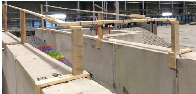
Figure D.8: The support construction for the measuring the slope.
