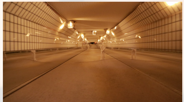
Figure 5.2 A quick test of using fixed-angle mirrors to increase the brilliance. The large piece of mirrors on the lower part of the walls are the remnants of previous experiment in Chapter 4.
