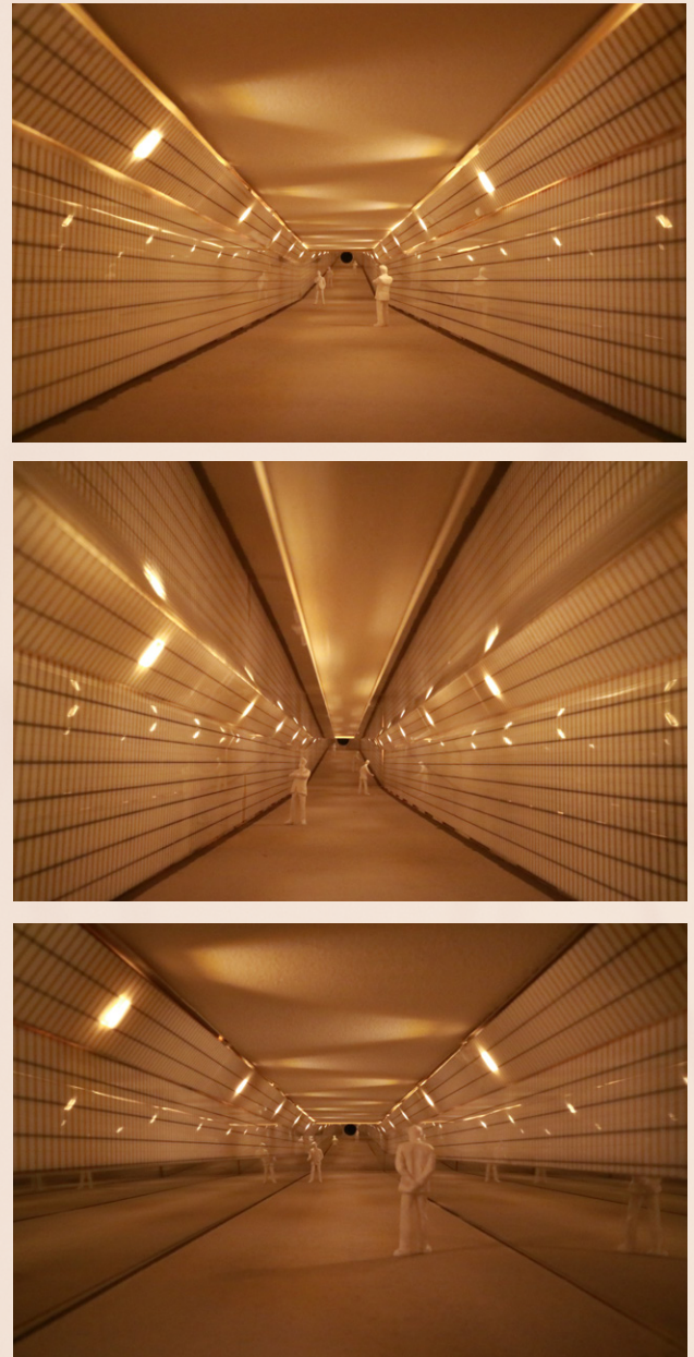
Figure 4.8 Scale models for observation test. From top to bottom is the original Maastunnel replicate, the CH tunnel and the CW tunnel. The black circle at the end of the tunnel is the reflected peephole
