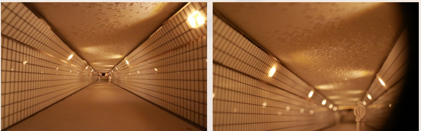
Figure 5.5 Photographs of scale model with glass beads creating RB on the ceiling. The glass beads are attached to the ceiling with spray glue.
