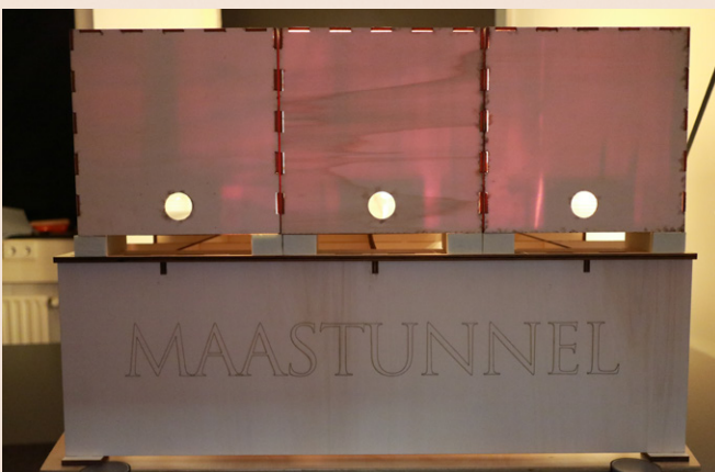
Figure 4.9 Settings of the scale models of Maastunnel for observation; in front view (a), the original Maastunnel replicate is in the middle, and the left and right one are CW and CH, respectively. In side view (b), the glowing part is the excess lighting of the models which was covered during the official observation session.
