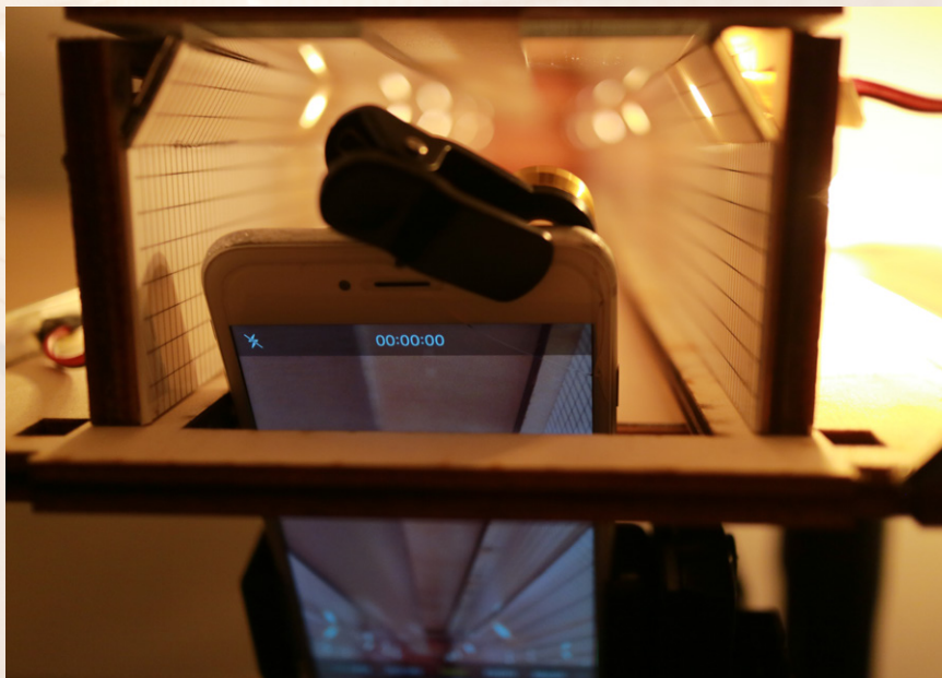
Figure 6.6 The track setting for the filming of the scale model. Note that the moving part is the whole tunnel, not the camera, which was not discernable to all the observers.
