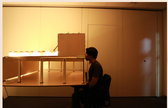
Figure 4.9 Settings of the scale models of Maastunnel for observation; in front view (a), the original Maastunnel replicate is in the middle, and the left and right one are CW and CH, respectively. In side view (b), the glowing part is the excess lighting of the models which was covered during the official observation session.
