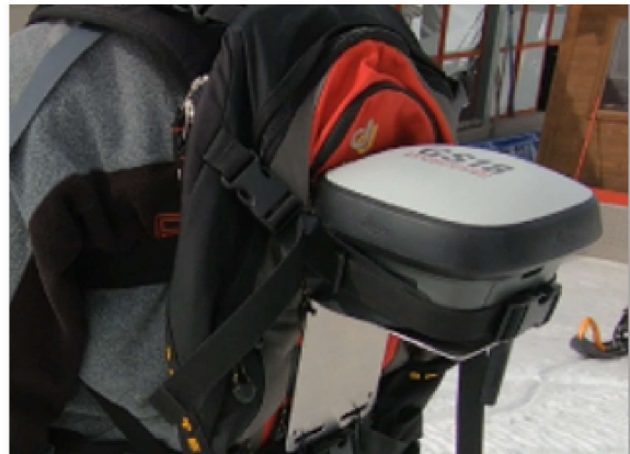
Fig. 3 The skier wore a backpack on which the position sensor was mounted. The sensor attached to a small aluminium plate which was secured to the backpack using straps.
