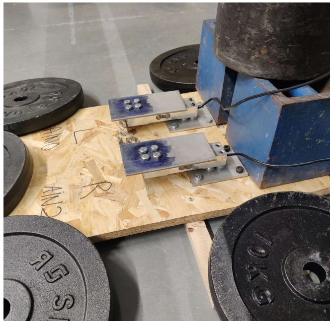
Figure D.4: The force plate that was created to validate the methodology of estimating the GRF by using IMUs. Two load cells are mounted on a wooden plate, which is kept at its place by heavy weights.
