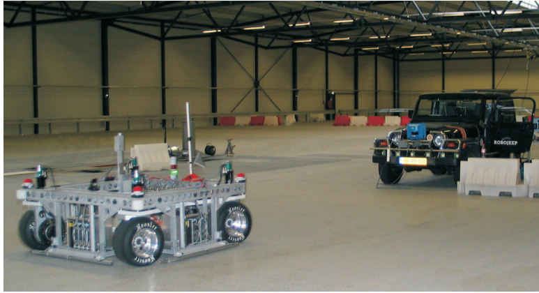
Figure 4.9: Experimental setup in VeHIL for sensor calibration with the moving base on the left, and the RoboJeep, equipped with lidar, radar and stereovision, on the right.
