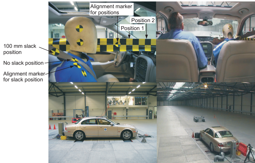
Figure 8.15: Experimental setup of a pre-crash test. Clockwise: dummy position with postures indicated; occupant view; moving base approach; side view.
