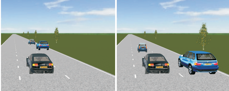
Figure 4.11: Visual representation of a cut-in scenario in the virtual world: an ACC-equipped vehicle drives on the middle lane, when suddenly one of the two preceding vehicles cuts in from the adjacent lane with a lower velocity.
