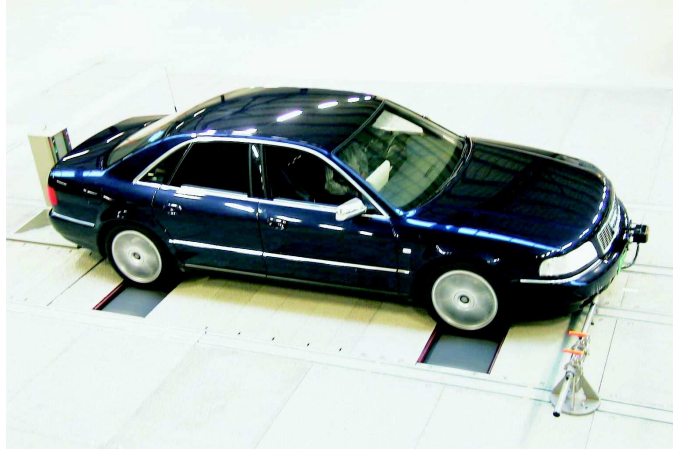
Figure 4.6: Vehicle under test with radar sensor at the front bumper, driving on the chassis dyno in VeHIL and supported by a rig at the front and back bumper.
