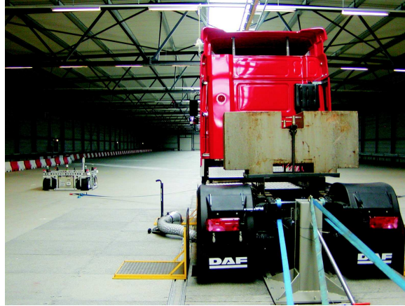
Figure 4.16: Experimental setup of a VeHIL test with a truck, equipped with an FCW system.
