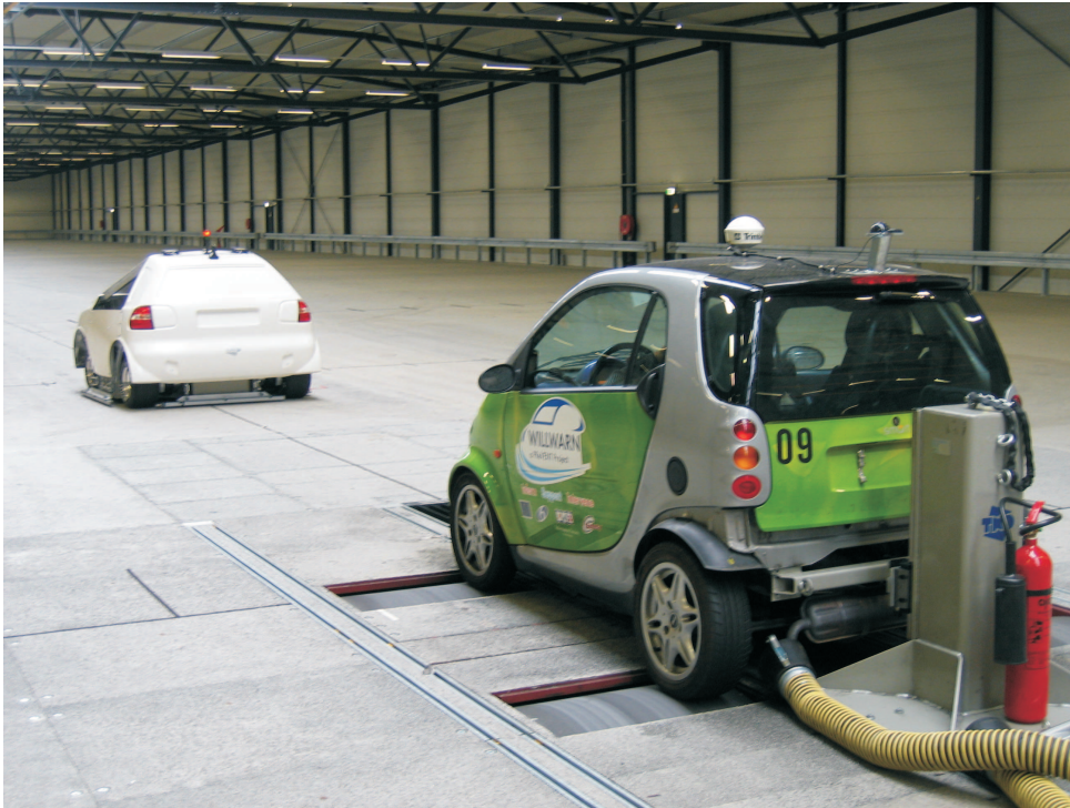
Figure 7.1: VeHIL laboratory setup: the Smart equipped with the CACC algorithm is following one of the moving bases.
