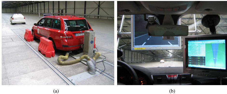
Figure 6.7: VeHIL laboratory setup: (a) the SASPENCE vehicle is set up on the chassis dyno (beneath the floor), and approaches another road user, represented by the moving base; (b) the real-time traffic scene is projected on a display in front of the camera system (located behind the rear-view mirror), while a preliminary HMI display shows the output of the SASPENCE system.
