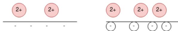
Figure 2.9: A visualisation of how discrete surface charge can lead to charge inversion. On the left: uniformly distributed surface charge, which is exactly screened by the counterions. On the right: discrete surface charges, which can cause overscreening.
