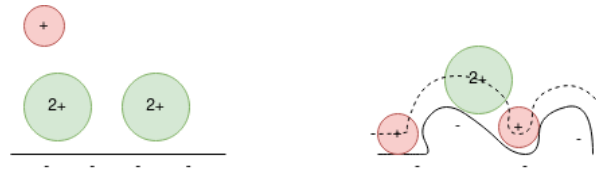
Figure 2.10: A visualisation of how surface roughness and ion specifics can contribute to ion competition. On the left, an example of adsorption on a flat surface. On the right, the bigger ion cannot access some of the spots on the amorphous surface. Note that the effect of hydration strength is not included.
