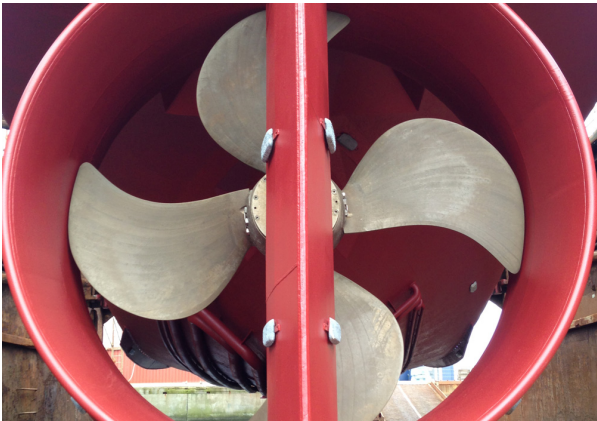
Figure 3.2: Controlable pitch propeller in a duct/nozzle [26]
