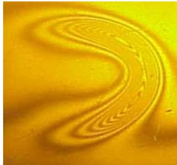
**Fig. 3.12** Newton fringe visualisation of the final spot from Figure 3.11. The spot has a width of approximately 3 mm.
