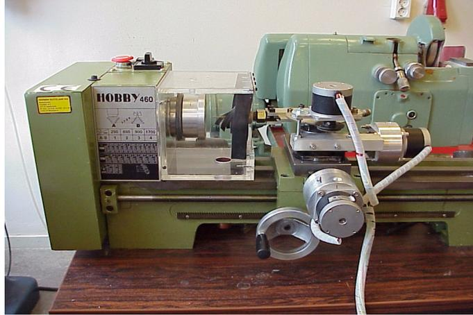
**Fig. 2.6** The bench lathe based FJP setup with the sample mounted on the left-hand side, the nozzle pointing towards the sample, in the horizontal plane, and the step engines that control the nozzle movement shown on the right.
