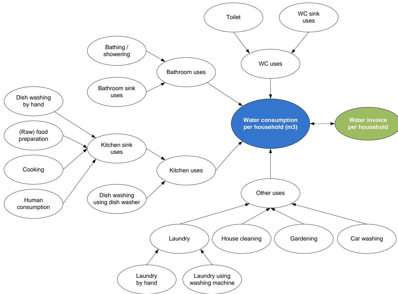
FIGURE 8 TYPICAL CONSTITUTION OF THE WATER CONSUMPTION OF A HOUSEHOLD
