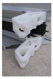
To the left: standard corner cleats made from aluminium profiles; to the right: AM corner cleats made from ABS plastic with the FDM technology.
