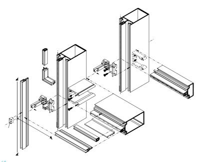
Figure 60 T-connector for orthogonal connection in AA-100 mullion and transom façade system by Alcoa; Imagery and illustrations from Kawneer-Alcoa digital catalogue, Issue 10/2010.
