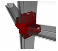
Figure 69 Principle of construction for façade node within a façade system; all angles can be digitally adjusted to the desired geometry and deformation.
