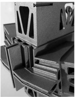
Printed nodal point in aluminium, realized on a ConceptLaser system by EOS @ FKM Sintertechnik GmbH
