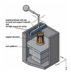
Figure 19 Schematic drawing: Poly]et™ method
