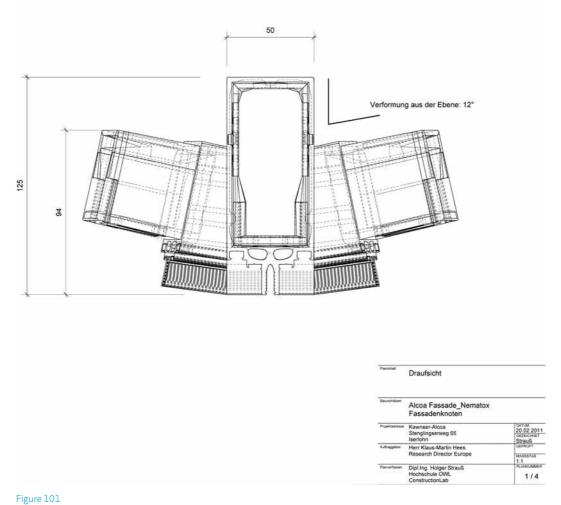
Technical drawing with real dimensions of the Nematox II; top view.
