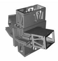
Figure 70 Rendering: NEMATOX II, 3D façade node for Alcoa 'AA-100' façade system.
