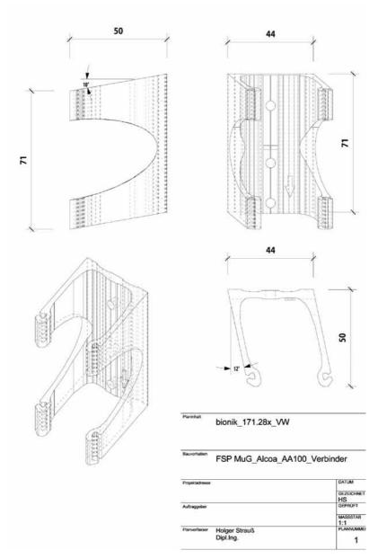
Optimised part as result of the optimisation for AM; in this part material was digitally 'cut off', where it is structurally not needed.
