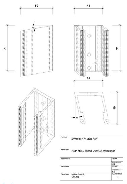
The first adjustment was the implementation of two different angles; this would allow for deformation in the façade.
