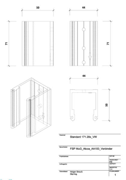
Figure 97 Technical drawing of the standard T-connector for a stick system; used as digital background for optimisation.
