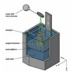
Figure 11 Schematic drawing: SLA method
