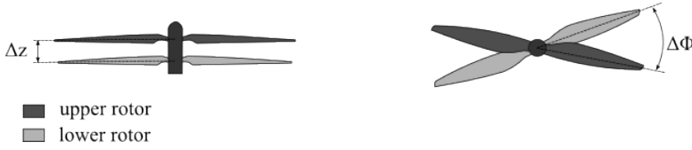
Figure 2.17: Co-rotating rotor geometry: \Delta x and \Delta\phi indicate the axial distance and azimuthal separation, respectively.
