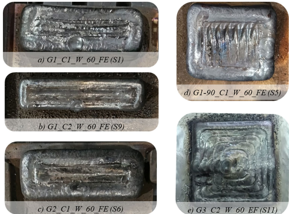
Fig. 8 Geometry of WAAM-fabricated components with rectangular (S1, S6, S9 samples) and square (S5, S11 samples) sections
