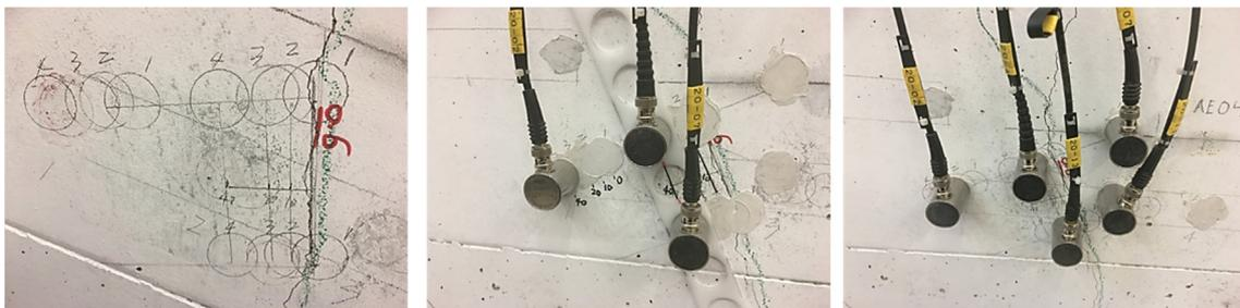
Fig. 5. Measurements on the influence of distance to crack (left and middle) and crack orientation (right).
