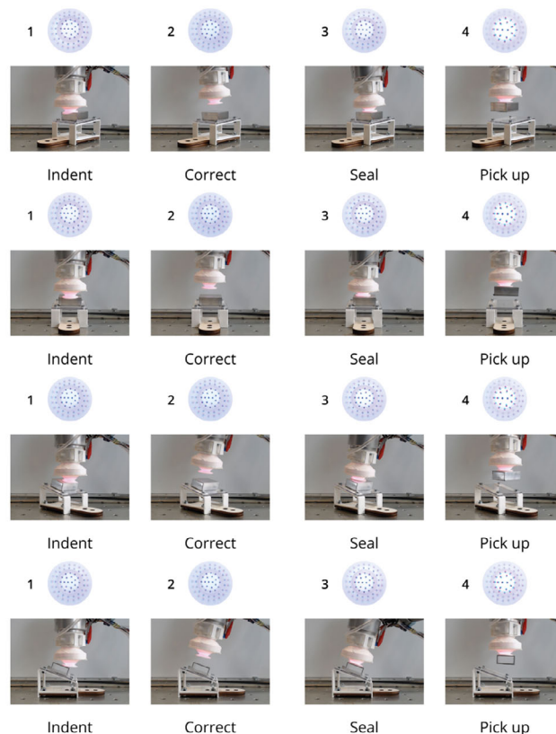
Figure 17. Performance of CNN when using it for live correction of orientation. For A) a latitude ( \theta ) of 5^\circ and a longitude ( \phi ) of 0^\circ , B) a latitude ( \theta ) of 10^\circ and a longitude ( \phi ) of 45^\circ , C) a latitude ( \theta ) of 15^\circ and a longitude ( \phi ) of 90^\circ , D) a latitude ( \theta ) of 20^\circ and a longitude ( \phi ) of 135^\circ . The left portion of each subfigure shows the obtained difference image and predicted values. The right portion shows the front view and tactile images in the 1) “indented” stage, 2) “corrected” stage, 3) “sealed” stage, and 4) “picked up” stage.
