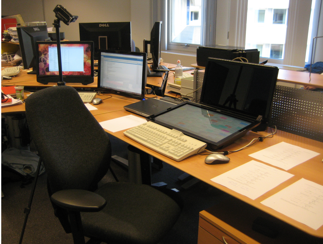
Figure 6.1: The setup used for the evaluations consisted of one touch screen, a laptop and a camera on a tripod to record the hand movements and comments of the participants. The papers to the right of the screen show the gestures and their corresponding actions.
