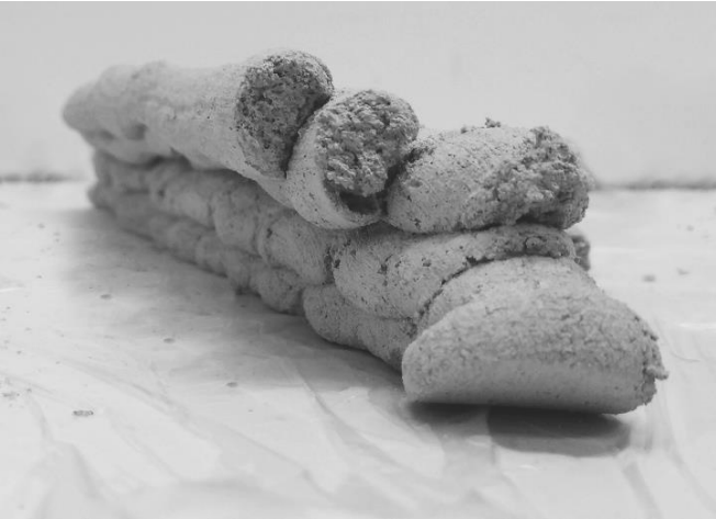
Fig. 41: stacked layers with laid down extrusion and 60+° overhang.
