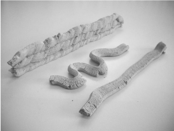
Fig. 38: rectangular nozzle, linear and S-shape single layer, stacked layer extrusion.
