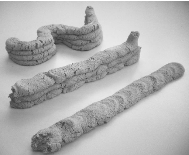
Fig. 39: Mixture 6 extruded on the print surface. single layer, stacked layer linear. stacked layer S-Shape.
