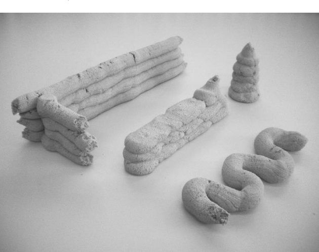
Fig. 40: S-Shaped laid down single layer, stacked linear layers extruded on the printing surface, stacked laid down extrusion, tower extruded on print surface.
