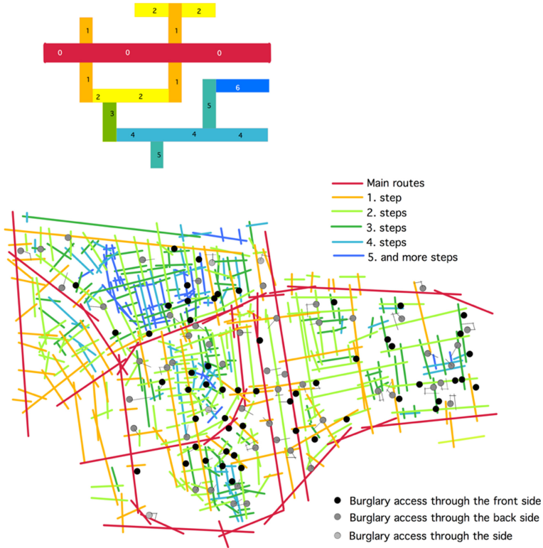
Fig. 2. How to calculate step depth from the main routes (top) and the analyses of the step depth from main routes with the dispersal of burglaries in the Dutch town of Gouda (bottom)
