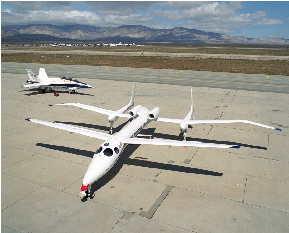
Figure 2.4: The Scaled Composites Proteus Optionally Piloted Aircraft with the OASys radar system under the nose and NASA's F/A-18 used for the flight tests; image courtesy of NASA, www.nasa.gov
