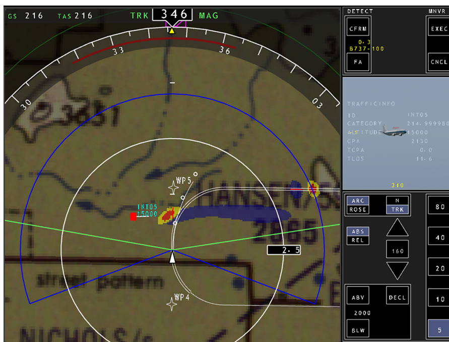
Figure 2.1: Screen dump of the CDTI display as shown to the operator
