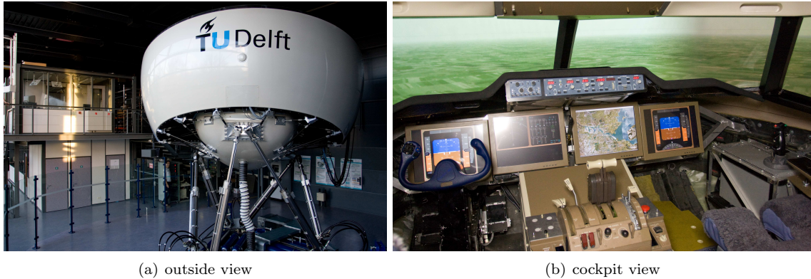
Figure 11. The SIMONA (SIMulation, MOtion and NAVigation) Research Simulator (SRS) at Delft University of Technology, source: Joost Ellerbroek
