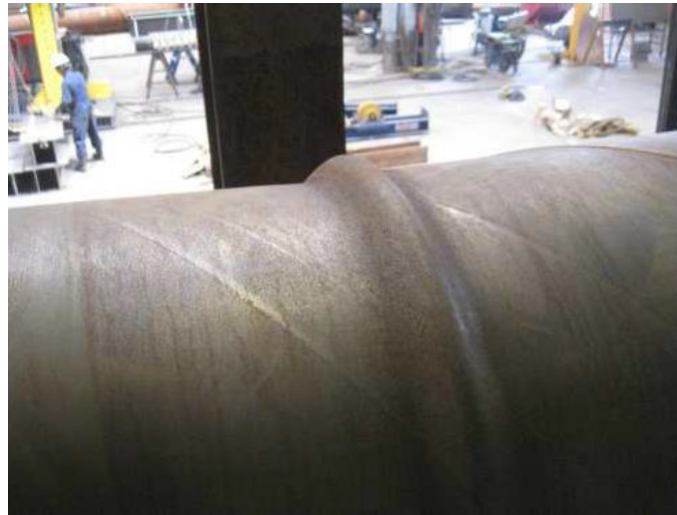
Figure 2.14: Typical buckling shape of sand-filled pile. [16]
