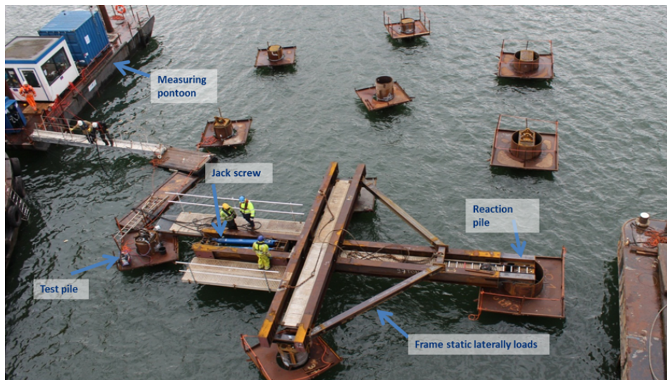
Figure 6.3: Top view of test set-up with static loading frame. [18]
