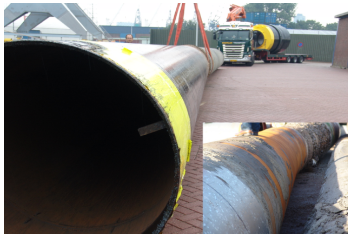
Figure 6.12: Permanently curved dolphin pile. [18]
