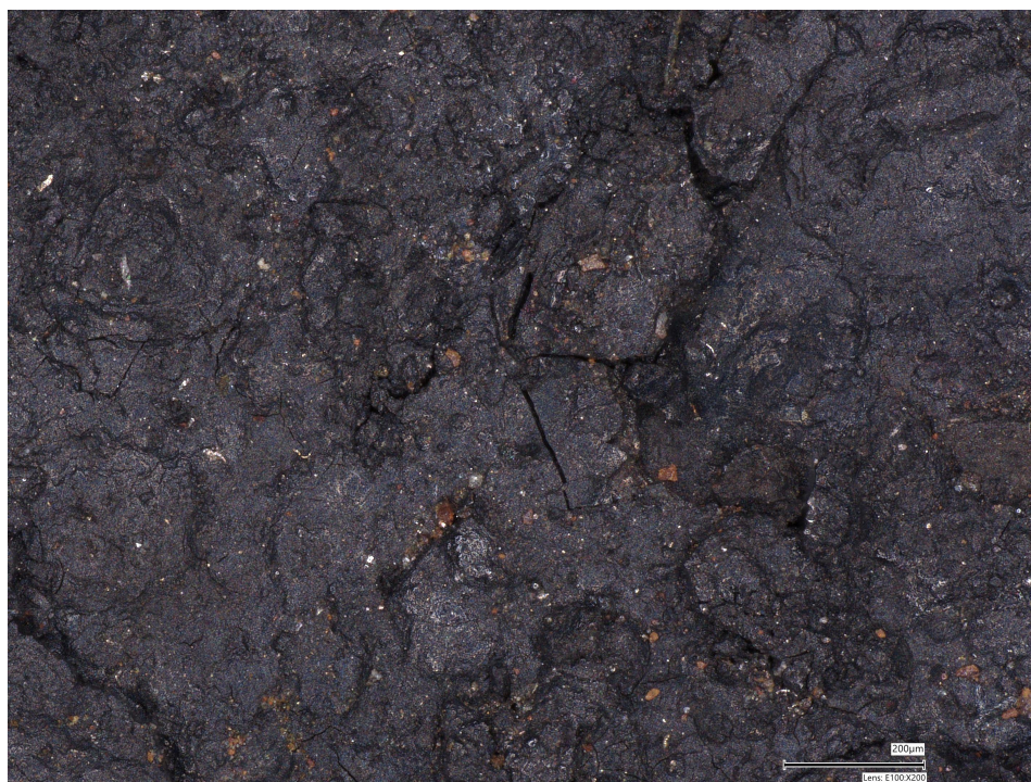
Figure 4.45: Post-charging oxide layer surface at 200x magnification.
