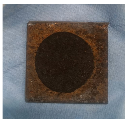
(b) X65 Oxide sample surface post-hydrogen charging.
