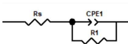
Figure 4.30: EEC model utilized for representing the electrochemical response of X65 Bare sample in 0.1 M NaOH + 3 g/L \text{NH}_4\text{SCN} .
