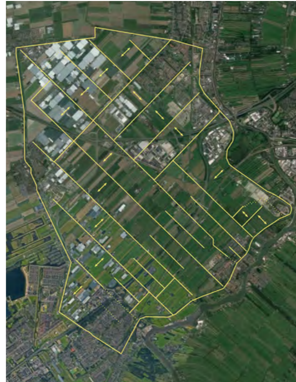
Fig. 16. Aerial picture of the Zuidplaspolder (Google maps) with overlay of the 1850 plan of the drained Zuidplaspolder (see fig.14).
