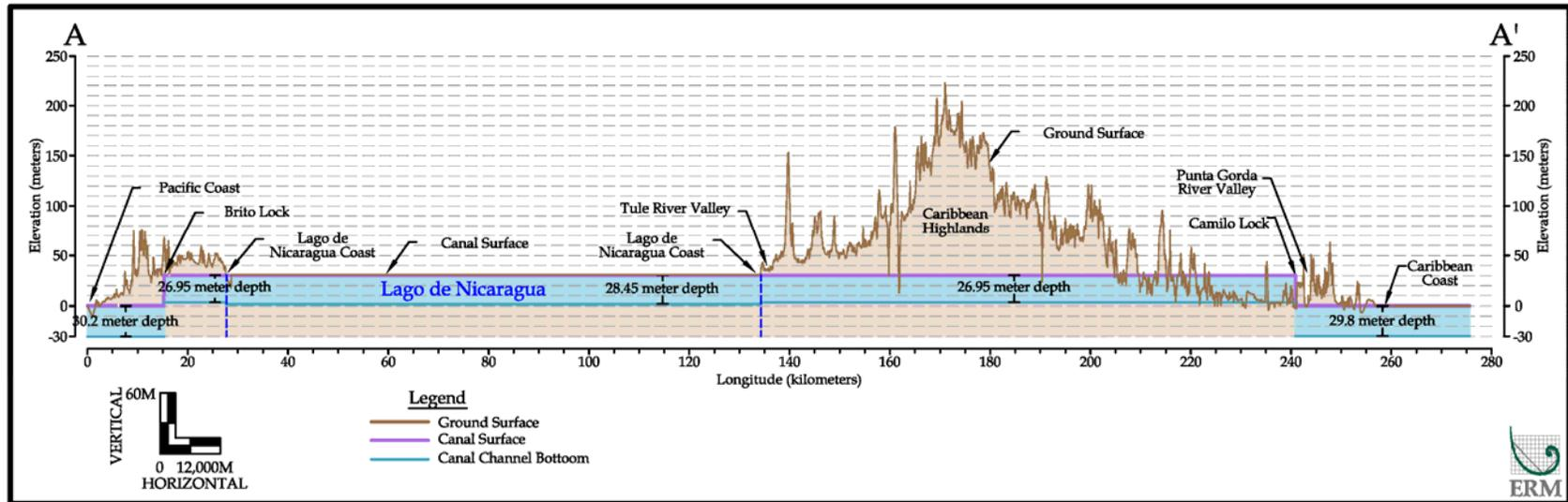
Figure 2-2: Canal Cross Section (200 Vertical Exaggeration)
