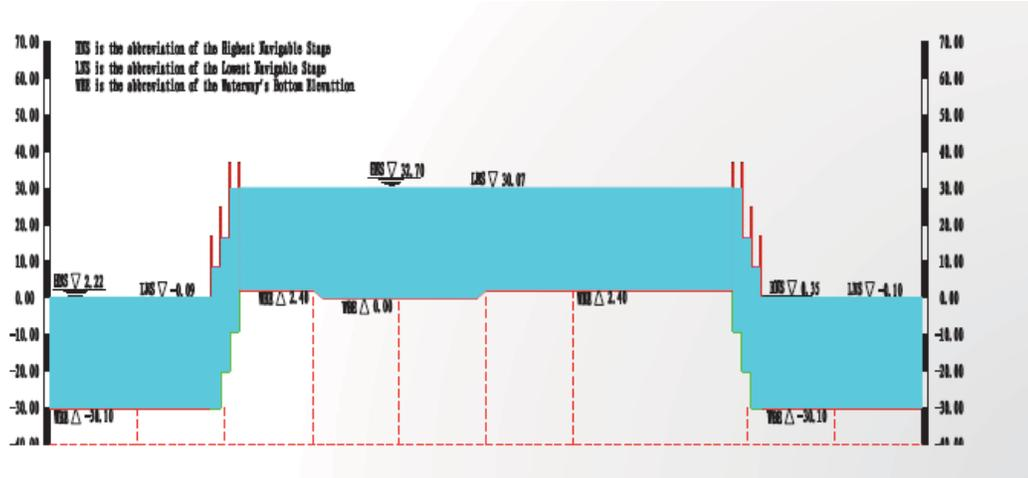
**Figure 3.1-3: Schematics of Water Level Change**
