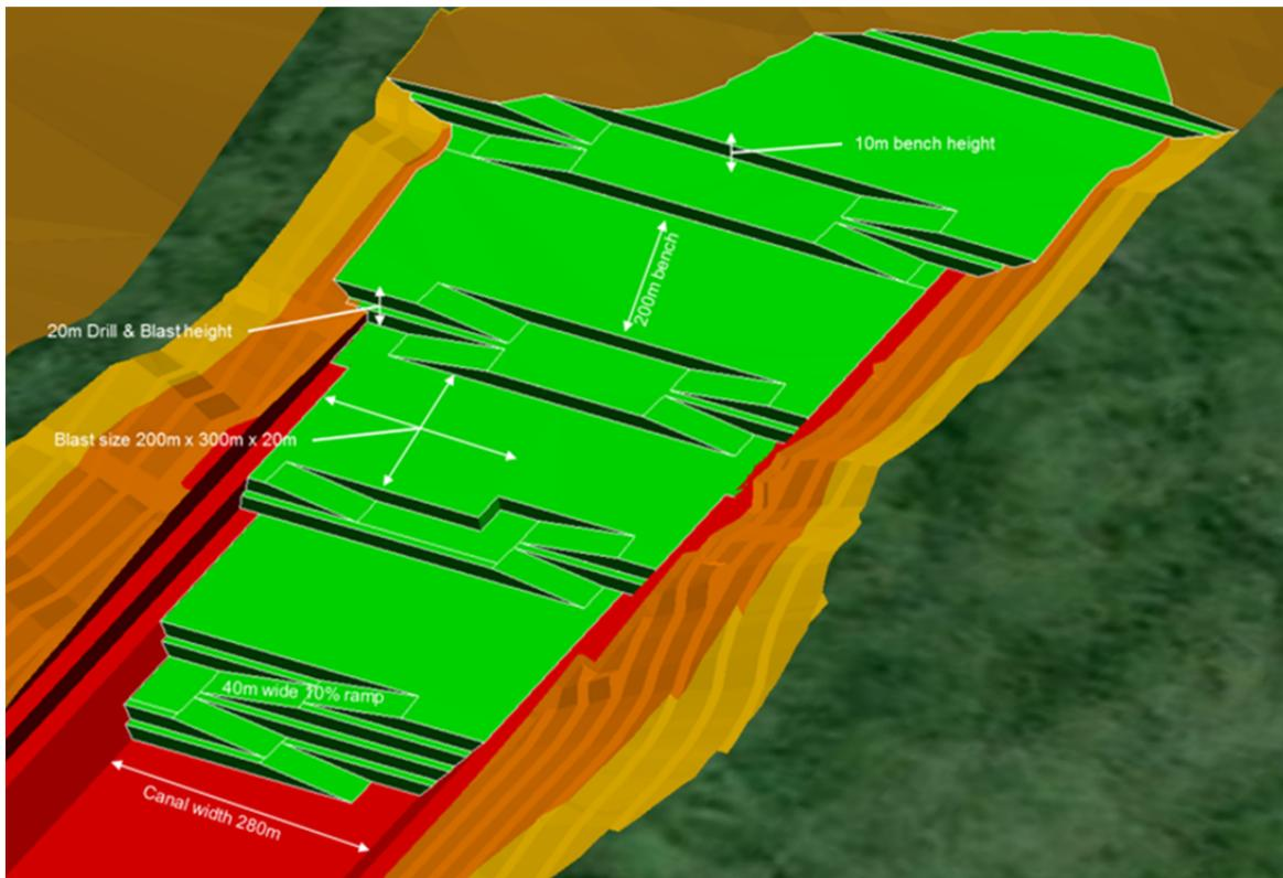
**Figure 4.6-6: Graphic of Benched Excavation within Canal Footprint**
