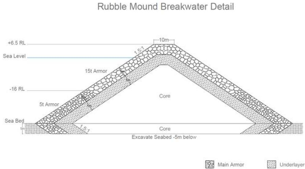
**Figure 3.1-15: Typical Cross Section of the Breakwater Structures**
