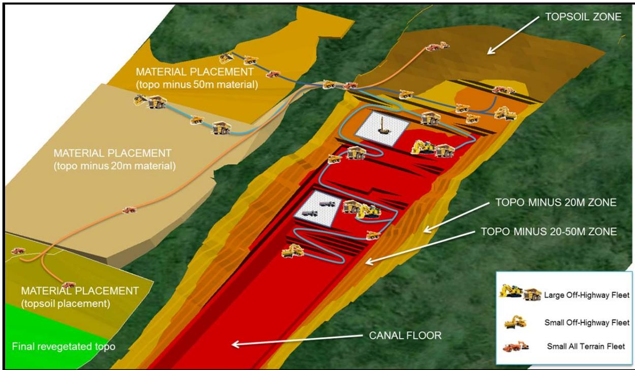
**Figure 4.6-8: Excavated Material Placement**
