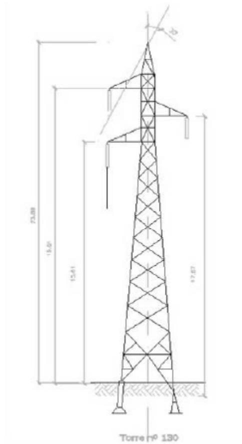
**Figure 3.3-4: Proposed Electrical Transmission Towers**
