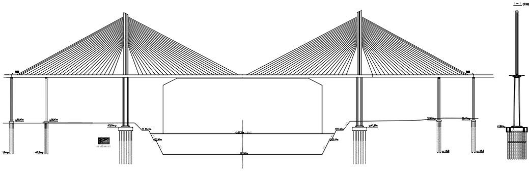
**Figure 3.3-1: Proposed Pan American Highway Cable-Stayed Bridge Profile**
