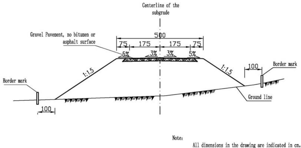
**Figure 3.3-3: Cross-section of Maintenance Road**
