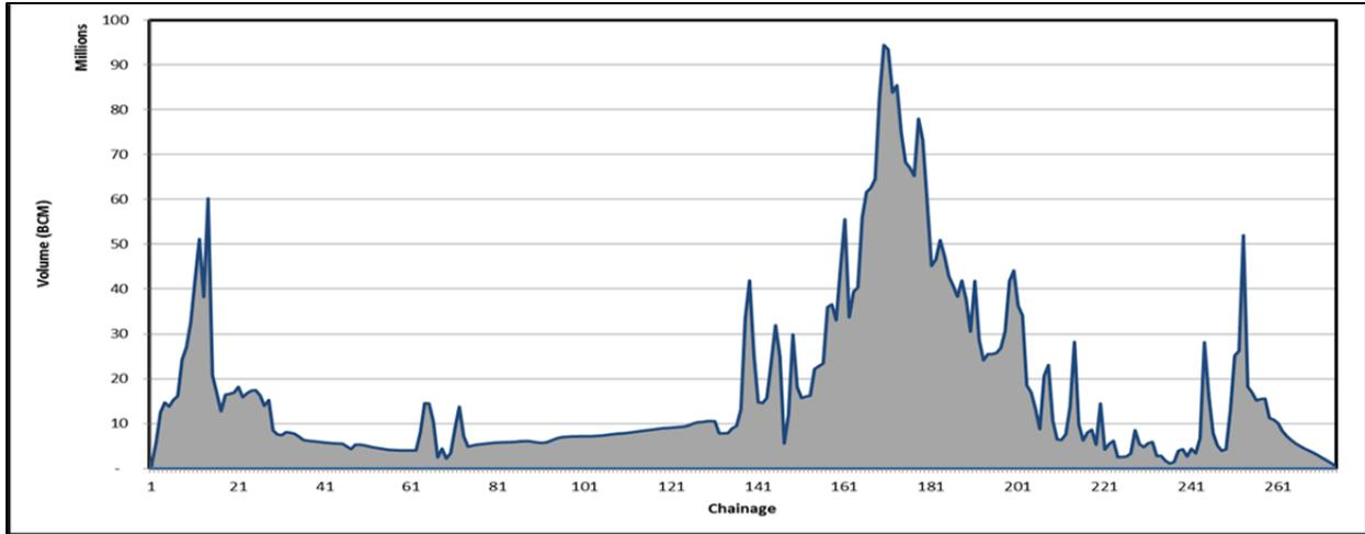
**Figure 3.1-9: Canal Excavation Volumes by Station**
