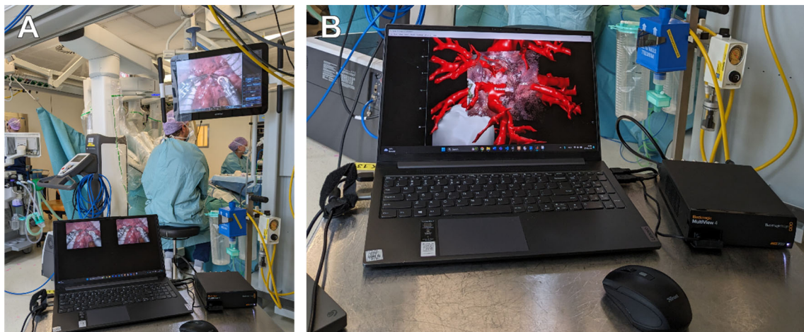
Fig. 2 Recording setup. A We used the Blackmagic MultiView 4 and Elgato Cam Link 4 k to record both the left and the right eye of the stereoscopic camera simultaneously. B Intraoperative augmented reality overlay using our proposed AR lung application. The overlay can
