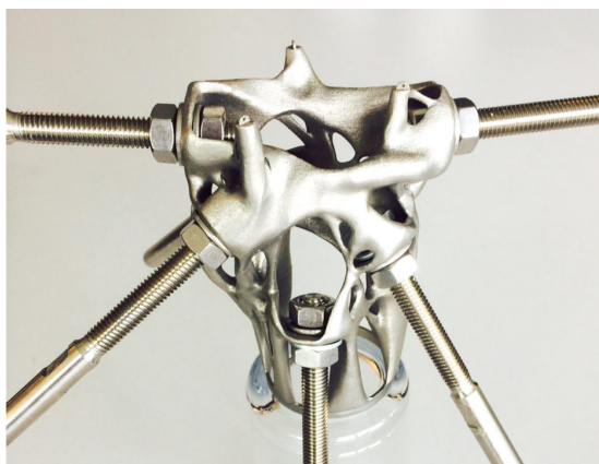
Figure 1.3: Stainless steel node made by additive manufacturing [9].
