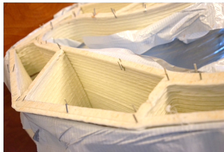
Figure 7.12: Staples at the bottom of the moulds.
