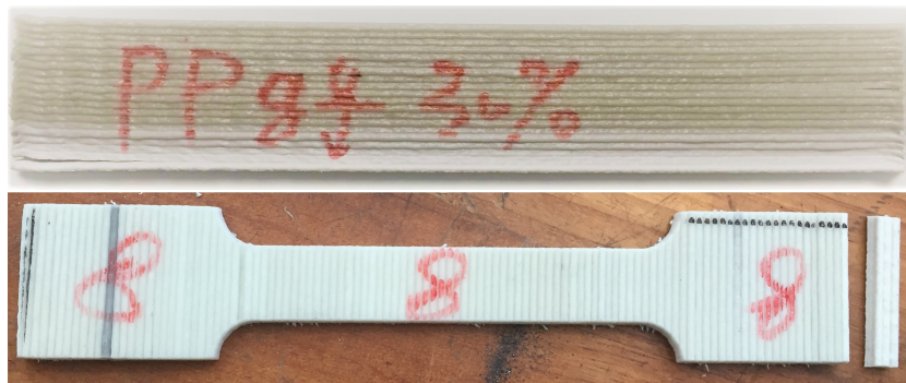
Figure 4.3: The influence of first printed layers. Up: the first printed layers in the printed product. Down: the failure at clamps.
