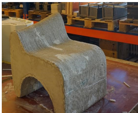
Figure 7.18: Final concrete product cast by the mould Part A .
