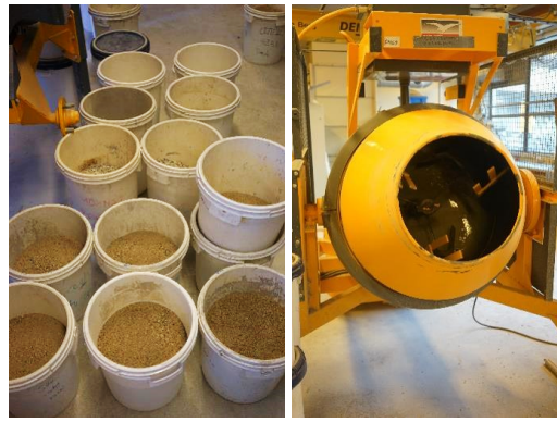
Figure 7.16: Preparation for the casting. Left: ingredients for the concrete mixture. Right: blender which has a maximum volume of 200 litres.
