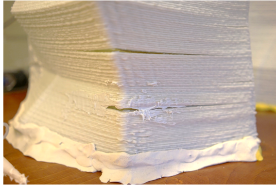
Figure 7.19: Double-curved part on the moulds where has cracks.
