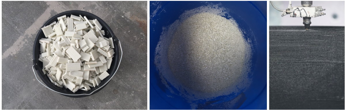
Figure 1.10: Preparation of the material for recycling at Aectual. Left: small segments. Middle: shredded pellets for printing. Right: printing process(example) [28].
