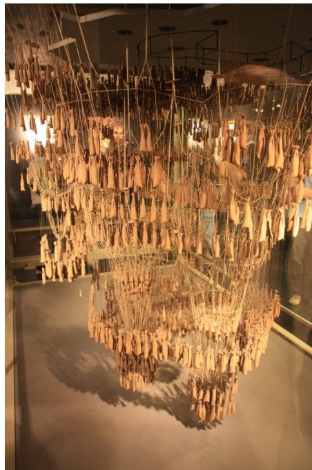
Figure 1.11: Form finding used by Antoni Gaudí during the design of Sagrada Família [29].
