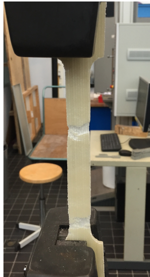
Figure 3.6: Plastic deformation with narrowing while testing Technomelt 3D 6910.
