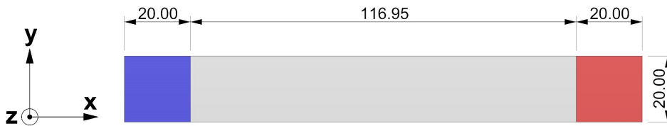
Figure 5.21: Numerical model for tensile test [mm]. Blue: clamped. Red: displacement in positive x direction.
