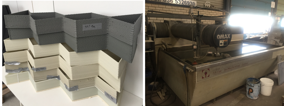
Figure 2.3: Preparation for the samples. Left: Printed geometry for preliminary test. Right: Water cutting machine at Schrijver B.V.
