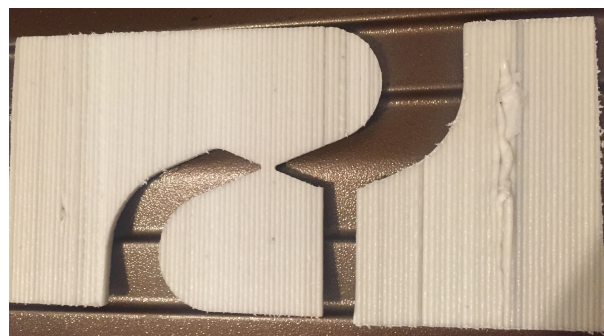
(b) Tensile failure at other location.
