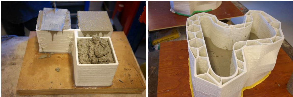
Figure 7.17: Casting process. Left: cast three cubes. Right: cast the mould.
