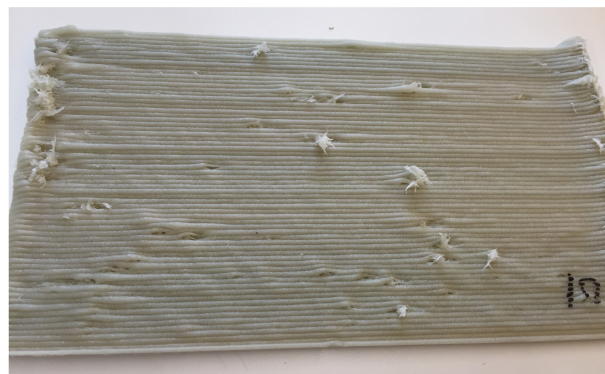
Figure 3.11: Bad quality of sheet of Technomelt 3D 6910 with multi-round printing
