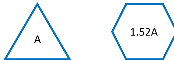
Figure 5.17: Area coverage of regular triangle and regular hexagon with the same perimeter. If the regular triangle covers an area of A , then the regular hexagon can cover 1.52A
