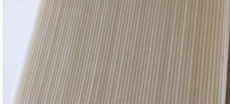
Figure 3.15: Decent printing quality with Technomelt 3D 6910.
