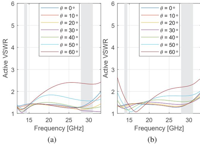
Fig. 5. Active VSWR for scanning up to  $60^\circ$  on the (a) E- and (b) H-plane.
