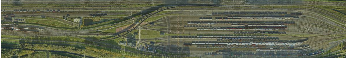
Figure 2.5: Aerial photo of Kijfhoek shunting yard. On the left is the arrival yard, then the wagons are pushed over a hump to the classification yard, which can be seen on the right. (Source: [4] )
