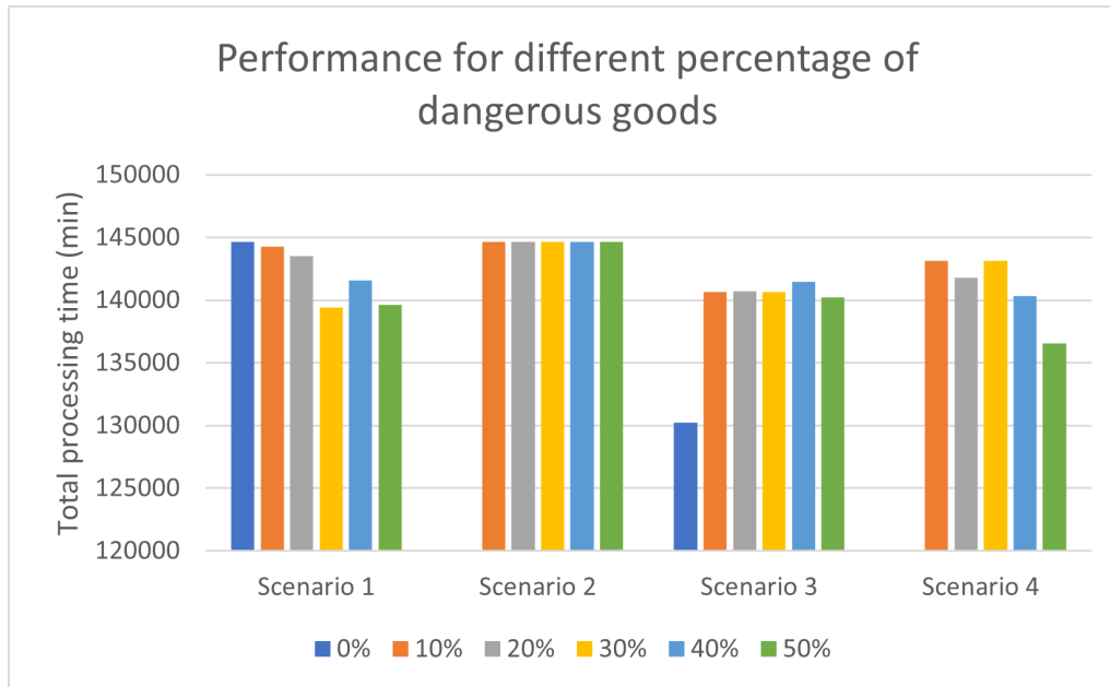
Figure 6.3: Results of sensitivity analysis for different percentage of dangerous goods, starting from 0 to 50%
