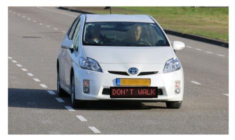
**Fig. 5.** eHMI concept 'DON'T WALK' in red letters overlaid over the photo. The person in the driver seat provided written consent for the publication of this photo. (For interpretation of the references to color in this figure legend, the reader is referred to the web version of this article.)
