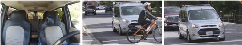
A cyclist is seen from inside the car; the car stops at zebra crossing; the light bar moves outwards and inwards while the cyclist crosses the road, after which bar centralizes, flashes four times, and becomes static when the car starts moving again (Ford Media Center, 2017)
