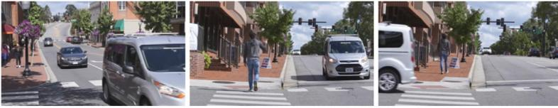
Bar moves inwards and outwards while the car approaches corner; the bar stabilizes in the center while turning indicator turns on, and a pedestrian crosses zebra intersection; the car turns into the corner (Ford Media Center, 2017)
