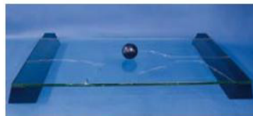
Laminated safety glass made of 2 x heat strengthened glass – top pane broken
