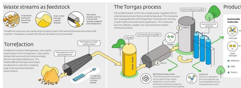
Figure 7: Working principle biomass-to-syngas plant through gasification and torrefaction [26]
