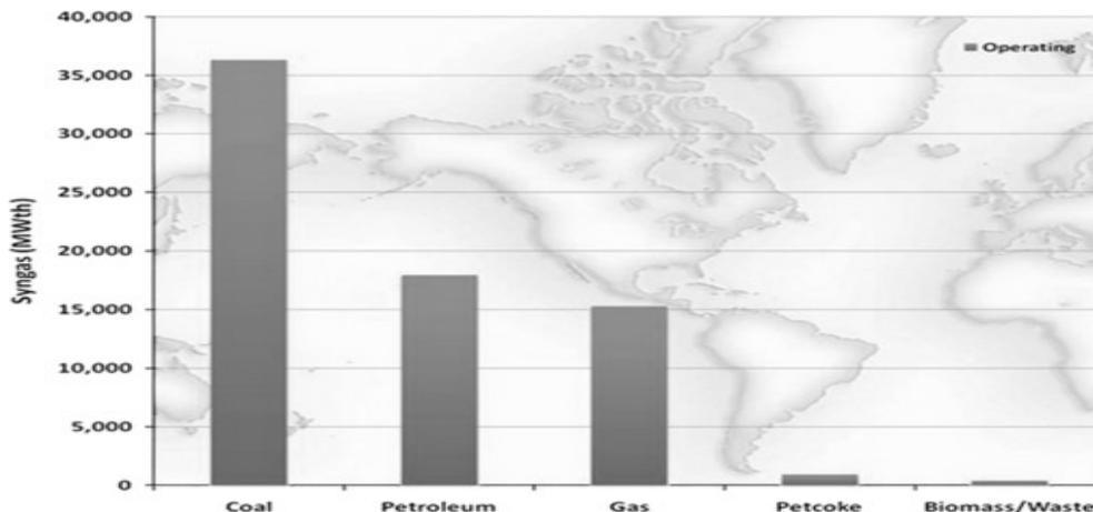
Figure 4: Overview of worldwide feedstock usage for syngas production [1]
