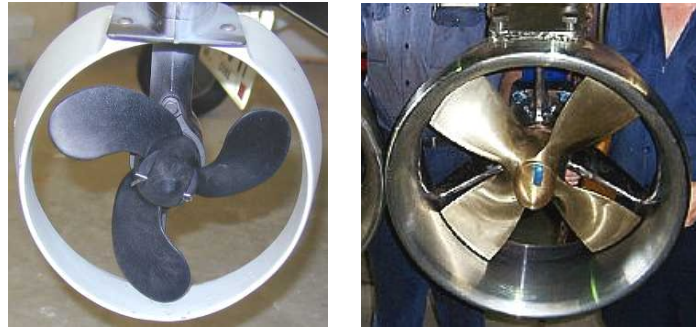
Figure 2-6: Ducted propellers with (left) traditional propeller blades and (right) Kaplan type propeller blades 3
