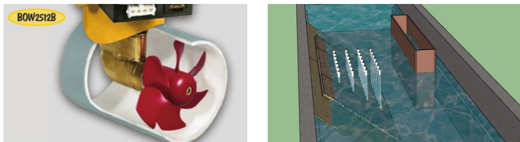
Figure 3-3: (left) The Vetus bow thruster type 2512B used by Van Doorn; (right) Basin geometry of Scenario 10 of Van Doorn
