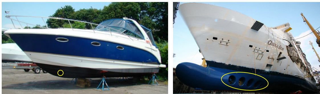
Figure 2-3: (left) A bow thruster in a small cruiser yacht; (right) Four bow thrusters in a very large cruise vessel. Both marked with a yellow circle
