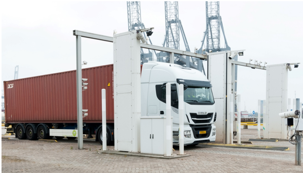
Figure 4.44: Fast Scan Vehicle and Container inspection system (“Douane Vervoer Controle” by Willem van Kasteren is licenced under CC BY-SA 4.0).
