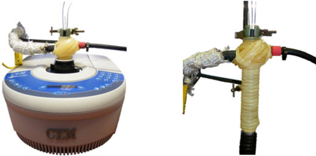
Figure 16. Microwave (l) and conventional (r) setup, each with the heated feed line on the left, temperature sensors coming out the top and the outlet on the right. Around the reactor, the oil tubing is visible.
