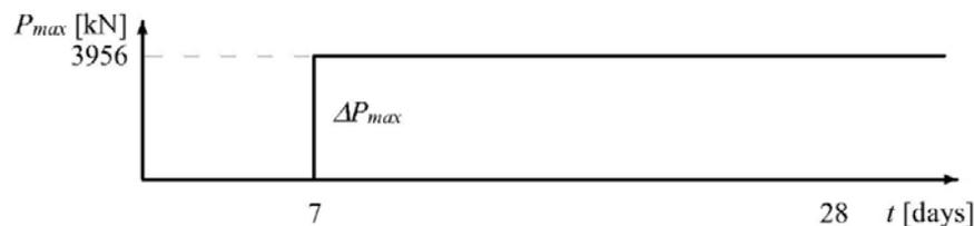
Figure 65: Prestressing Steps of New Decks.
