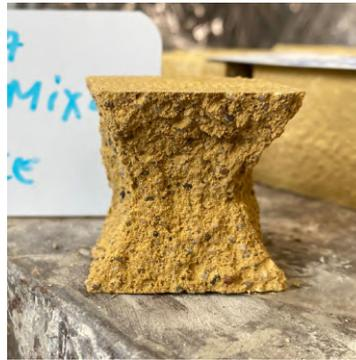
**(b) Artificial soil**
