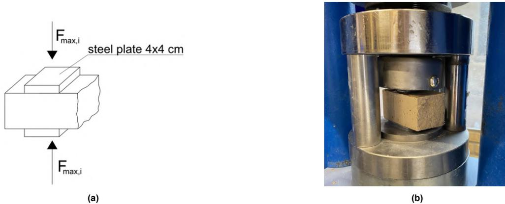
**Figure 6.6:** Determination of compression strength: (a) static scheme, loading, and geometry of tested specimens; (b) the view of the specimen ready to test.
