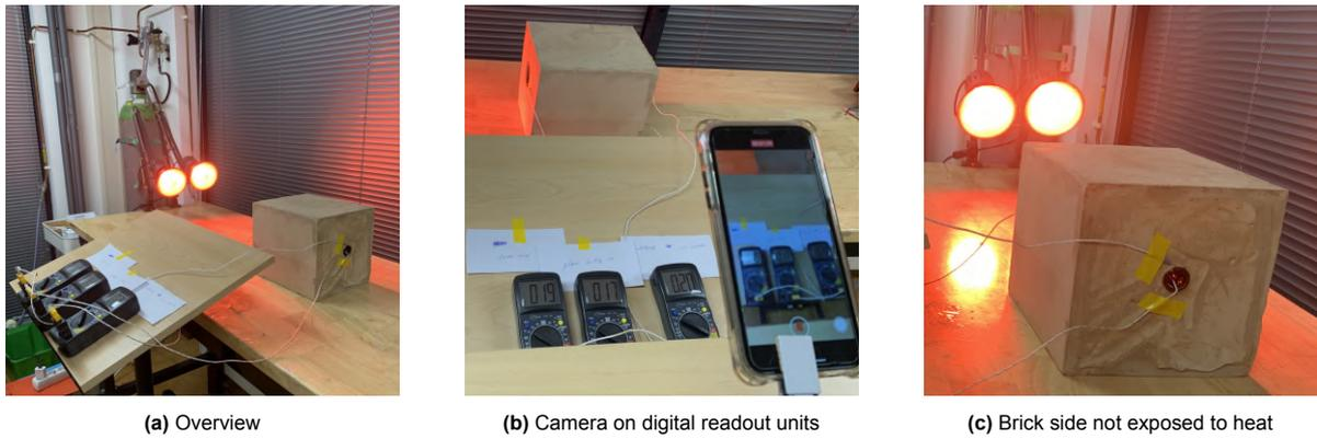
Figure 7.14: Test set-up: Sunlight Exposure
