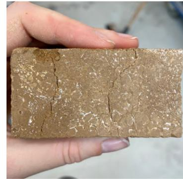
**(c) Natural soil****Figure 6.12:** Failure mechanisms earth based mortar
