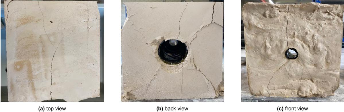
Figure 7.17: Crack Pattern Sample 1
