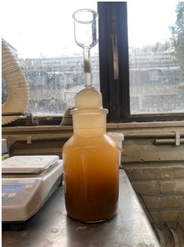
(a) Test set-up Pycnometer
