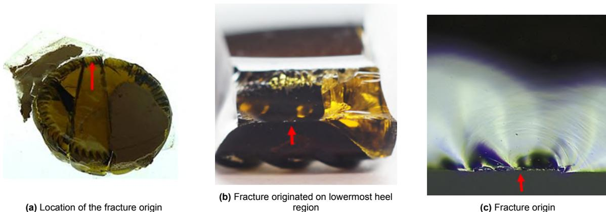
**Figure 7.6:** Location of fracture origin indicated with arrows: Sample 2
