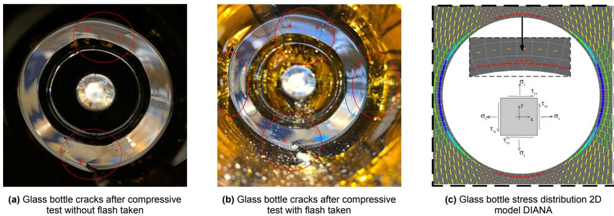
**Figure 8.22:** Comparative Analysis: 2D FEM Model versus Physical Compression Test Results
