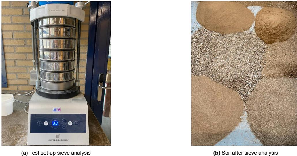
**Figure 6.2:** Sieve analysis Dutch soil originating from Emmen
