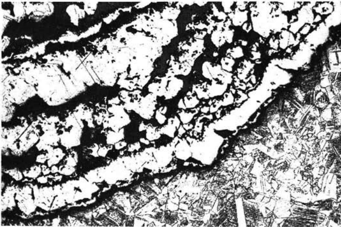
Figure 5.5.1. Plug type dezincification. a. schematic cross section; b. photograph of tube with plug type dezincification; c. photomicrograph of boundary between porous copper residue (upper left) and unattacked brass.
