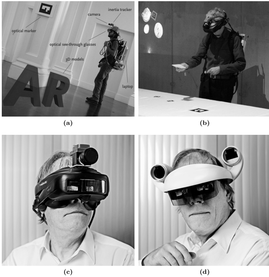
Figure 2.3: AR systems with optical see-through HMDs of Cybermind used in the Delft University of Technology in chronological order. The system shown in (d) is designed by ARlab student Niels Mulder.
