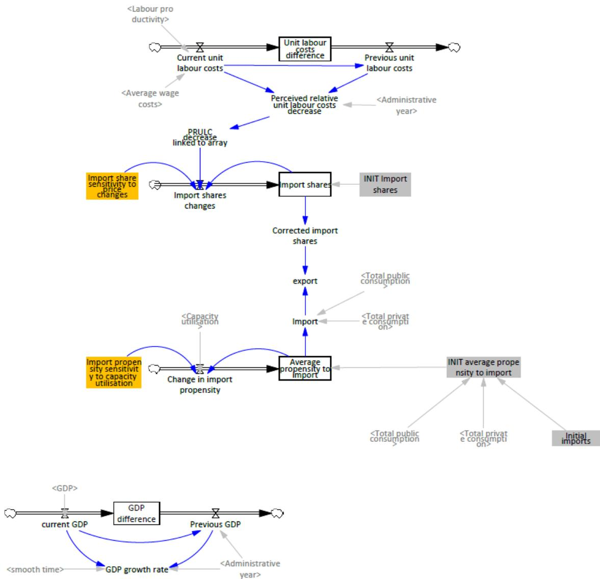
Figure 8.5 Stock-flow diagram of trade sub-model.
