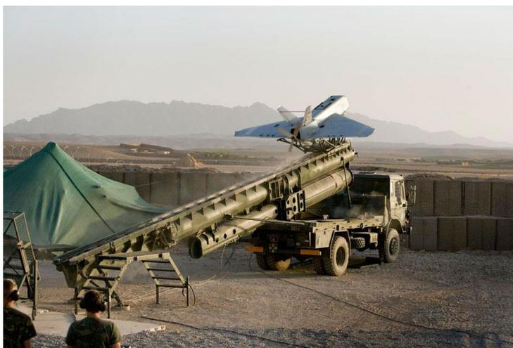
**Figure 17: Sperwer launching installation<sup>35</sup>**
