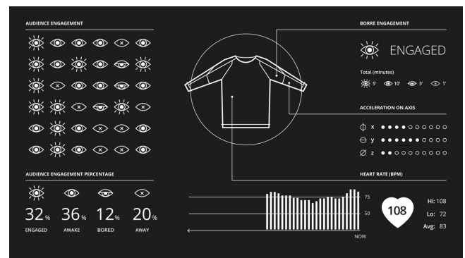
Figure 4. Visualisation showing audience engagement (left half) and sensor readings of the presenter (right half).
