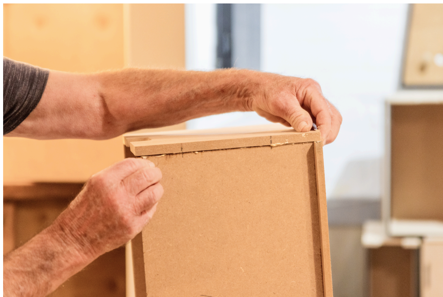
Figure 4.26 Placement of the front, fixed with biscuits and glue
