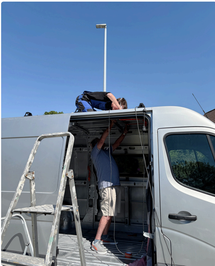
Figure 2.11 Author installing MaxFan
