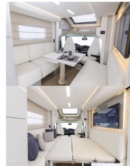
Figure 3: Camper Design from Brischetto et al. (2019) in daytime and nighttime configuration.
