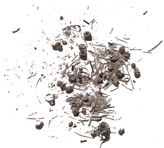
Figure 63: Silver bits retrieved from the samples used in the experiments. Approximately 2,1 grams.
