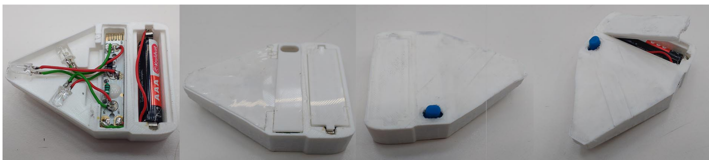
figure 4: a 3D printed casing for a bike light with covers that can be printed over to seal the product, but can be broken open to retrieve the parts. Part of the preliminary field study into design for non-destructive disassembly.
