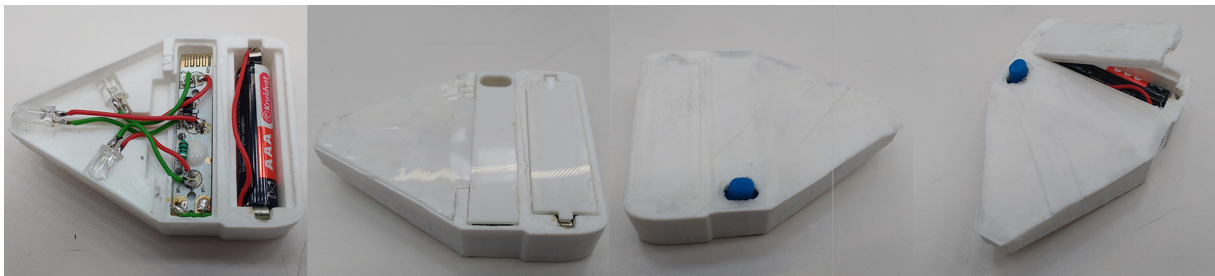
Figure 68: a 3D printed casing for a bike light with covers that can be printed over to seal the product, but can be broken open to retrieve the parts.
