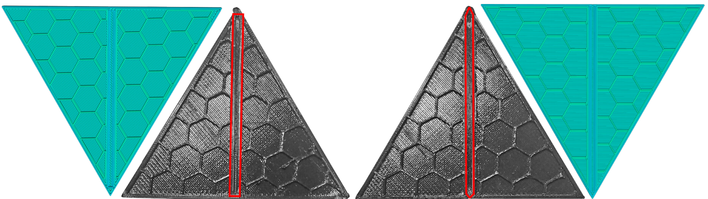
Figure 21: cuts in walls schematic slicer preview and photo's: left only in the bottom, right in the bottom and walls.
