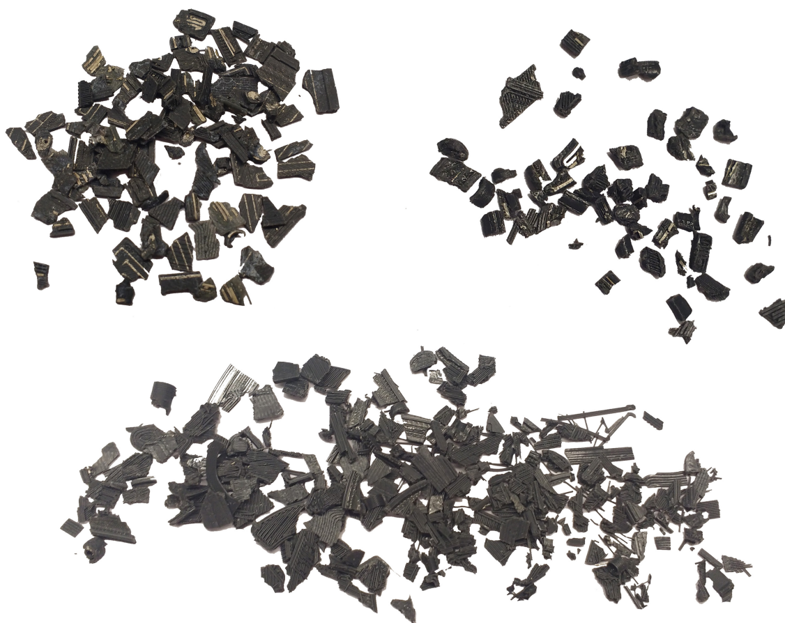
figure 5: fractions of middlings: shreds with a combination of dissimilar materials. Part of the preliminary field study into release of the silver from PLA substrate in a shredder.
