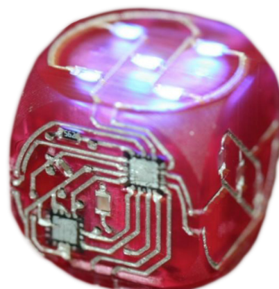
figure 2: prototype of a electronic gaming dice with embedded accelerometer, microprocessor, and LED's. (MacDonald et al.,2014)
