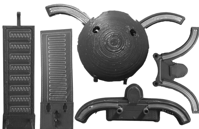
Figure 48: examples of used samples, 3D printed PLA and silver manufactured with a Voxel8 multi-material printer. Not to scale.
