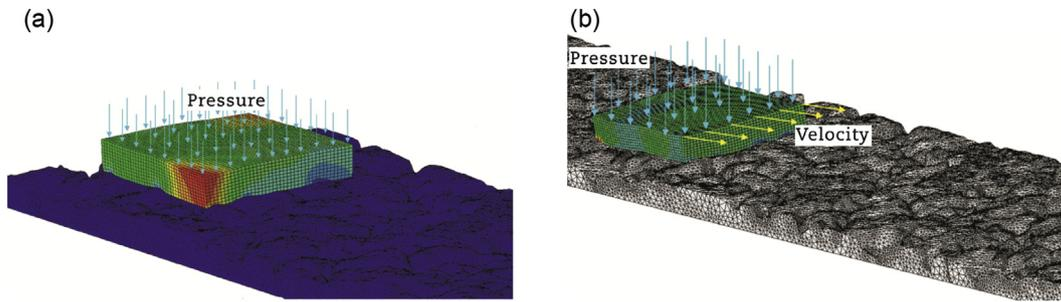
**Fig. 4 – Micromechanical simulation of interaction of rubber pavement morphology. (a) Indenting the rubber block onto pavement morphology. (b) Sliding the rubber block longitudinally over the pavement morphology.**
