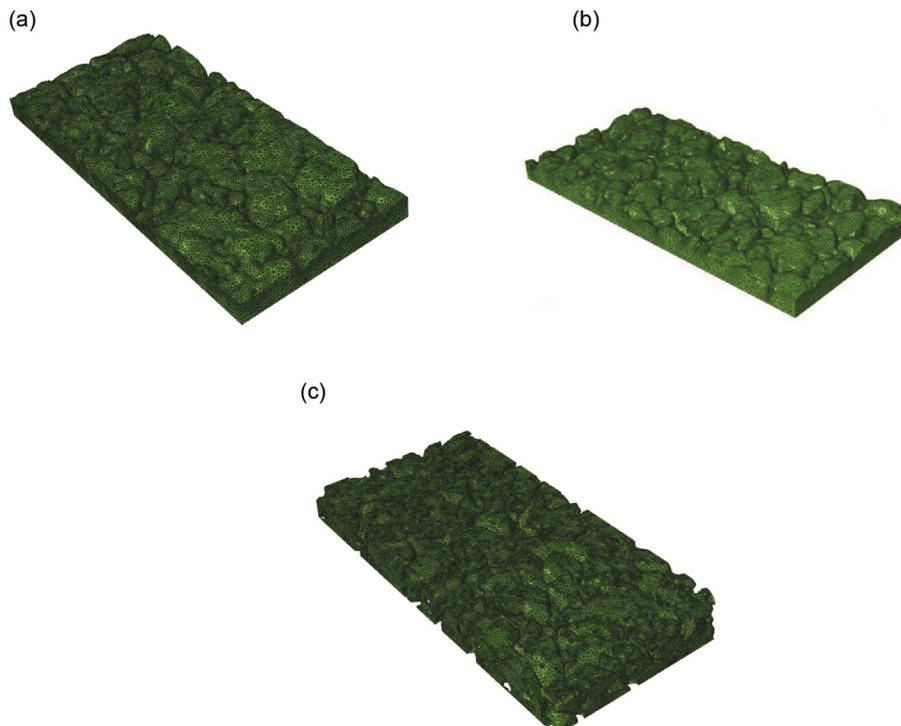
**Fig. 2 – 3D view of asphalt pavement morphology. (a) SMA rigid pavement. (b) UTS rigid pavement. (c) PA rigid pavement.****Table 3 – Mix compositions.**
