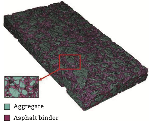
**Fig. 3 – 3D view of flexible UTS pavement morphology.**
