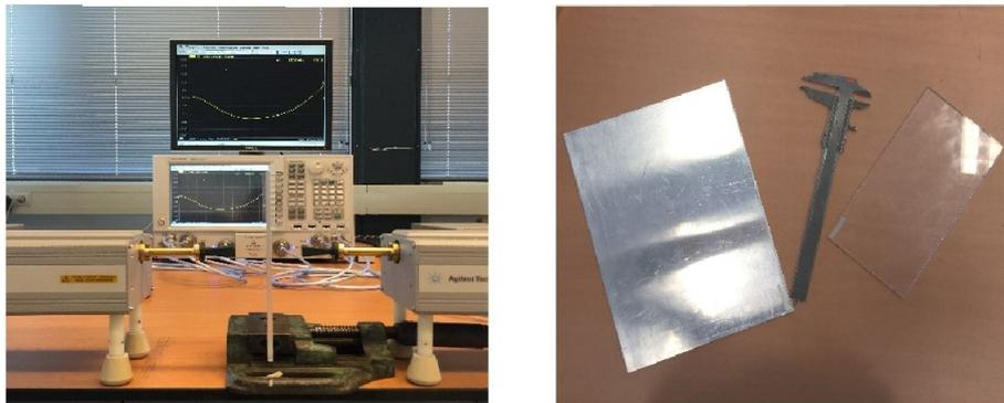
Figure A.1: Experimental settings for the measurements of the dielectric properties of the radome
