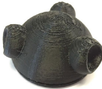
Figure 5 An example of a poor-quality 3D print finish occurring from the layering process on curvaceous surfaces. This is avoided by reorienting the product on the print bed.
