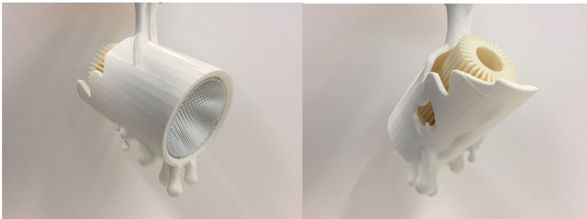
Figure 4 An example of one concept pushing the boundaries of organic 3D CAD modelling and exploiting the capabilities of 3D printing over injection moulding.
