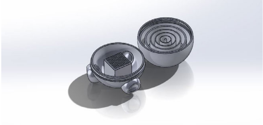
Figure 8 The CAD development of sample spheres used to better understand low-cost 3D printing capabilities with a focus on curvaceous forms.
