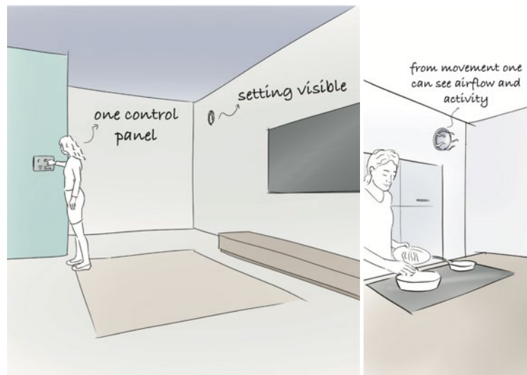
Figure 16 Using the supply valves to prove the system is working and show what it is doing.
