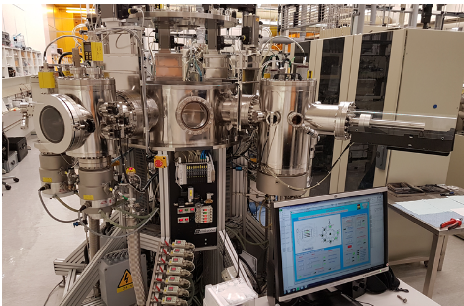
Figure 3.4: The Amigo PECVD cluster tool by Elettrorava S.p.A. with the control software running in front
